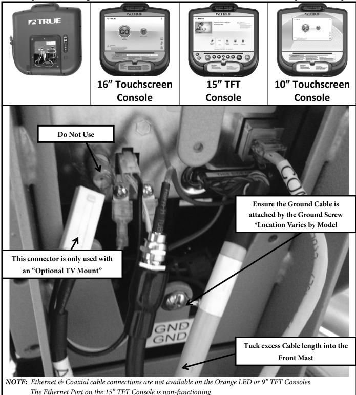
All Ground Wires Must be connected
