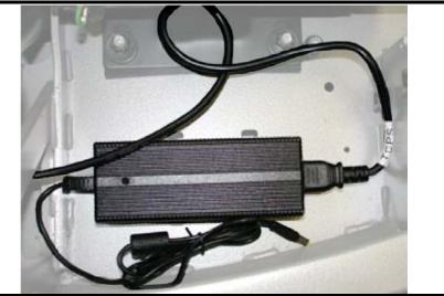
**d**) Separate the **AUXPS** cables that are attached to the **CNTRL** cable (coming from the bottom of the right pedestal) and cut the wire tie holding the female end of the **AUXPS** cable to the **CNTRL** cable as shown.
