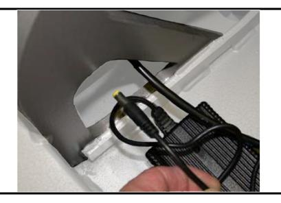
**e**) Route **AUXPS** Power Supply Cable from power supply through the cutouts in both incline tower plates as shown.
