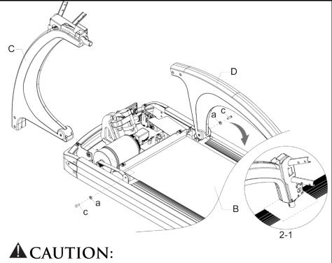
Pedestals can pivot until secured in front. Do not grab top of pedestal.
