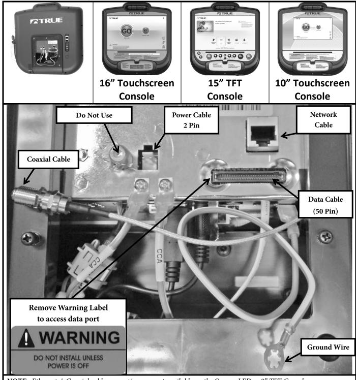
**NOTE:** Ethernet & Coaxial cable connections are not available on the Orange LED or 9" TFT Consoles The Ethernet Port on the 15" TFT Console is non-functioning **All Ground Wires Must be connected**
